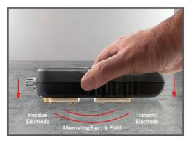
This field penetrates the material under test. The very small alternating current flowing through the field is inversely proportional to the impedance of the material. The instrument detects this current, determines its amplitude and thus derives the moisture value.
