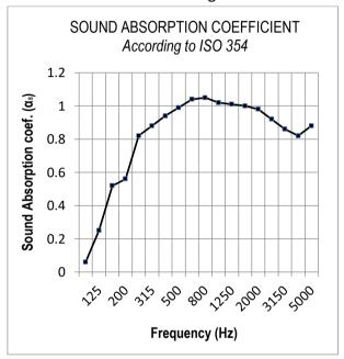
The Noise Insulation test data must be obtained in accordance to EN ISO 140.3 Acoustics – Measurement of Sound insulation in buildings and of building elements & rated the sound insulation in buildings elements according to EN ISO 717.1. The Sound Absorption coefficient should be measured in a reverberant chamber in accordance with ISO 354.
